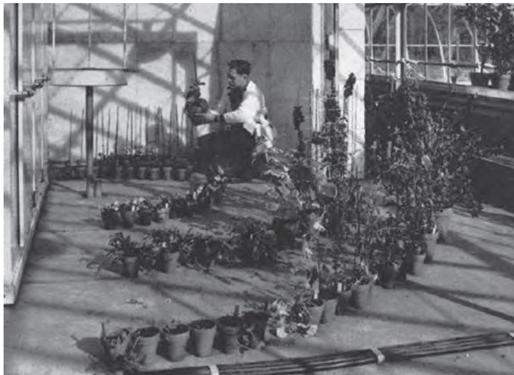
Fig. 4.27.1: Plants growing in the gamma greenhouse at Brookhaven National Laboratory. The plants are arranged in concentric rings around the radioactive ^{60}\text{Co} source, which is in the pipe extending into the floor (circa 1959) [220]. (Photo Source: Life Sciences Foundation (LSF) Magazine).
