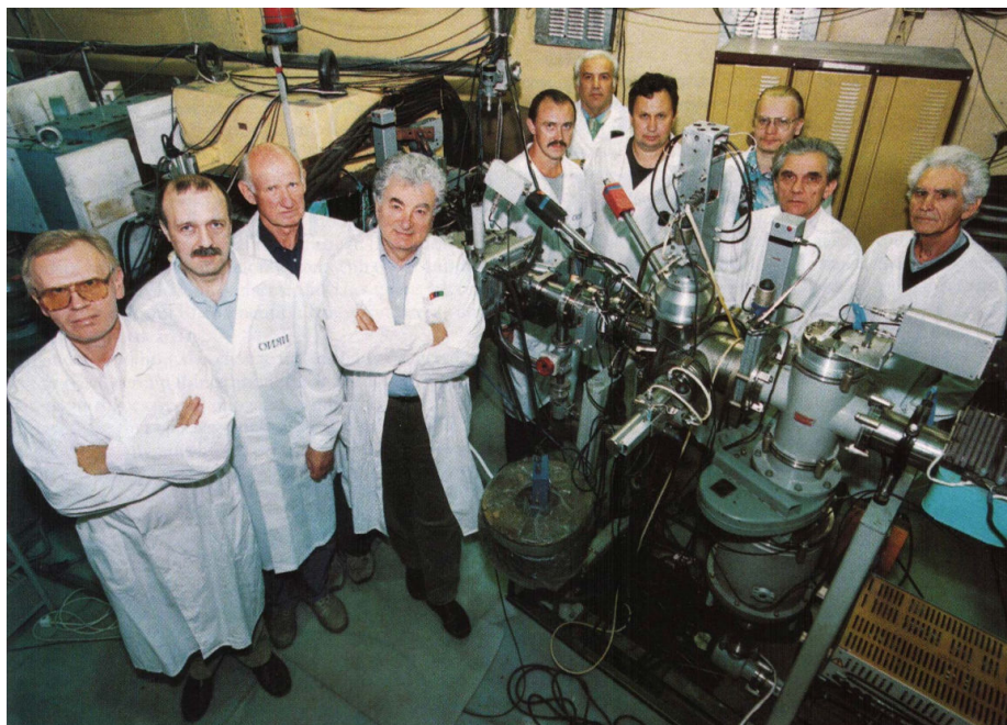
Fig. 4.114.1: The research team at the Joint Institute for Nuclear Research (JINR) in Russia that discovered flerovium with a team from the Lawrence Livermore Laboratory in the USA. They are standing around one of the mass separators that they use to produce superheavy elements . (Photographer: Yuri Gripas Gamma Liaison) (Picture Source: Yuri Ts. Oganessian, Joint Institute for Nuclear Research) [665, 667].
