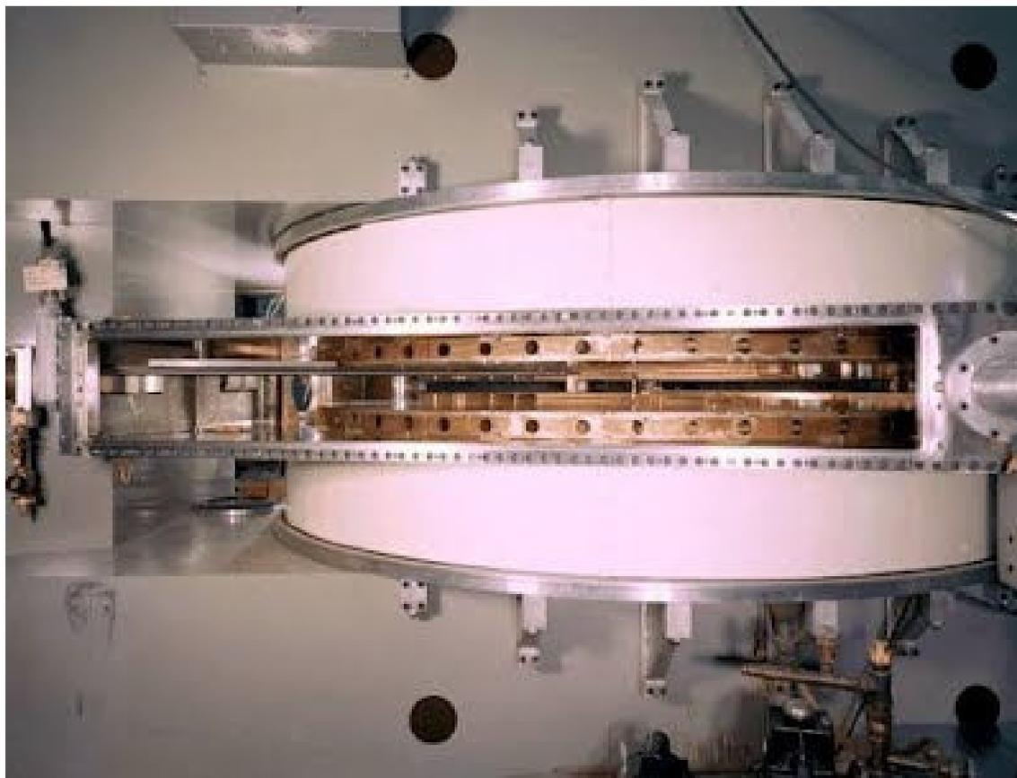
**Fig. 4.44.2:** The 88-Inch **cyclotron** was used to produce both light and heavy ions, including  $^{94}\text{Ru}$  and  $^{95}\text{Ru}$ . (Photo Source: Lawrence Berkeley National Laboratory) [333].
