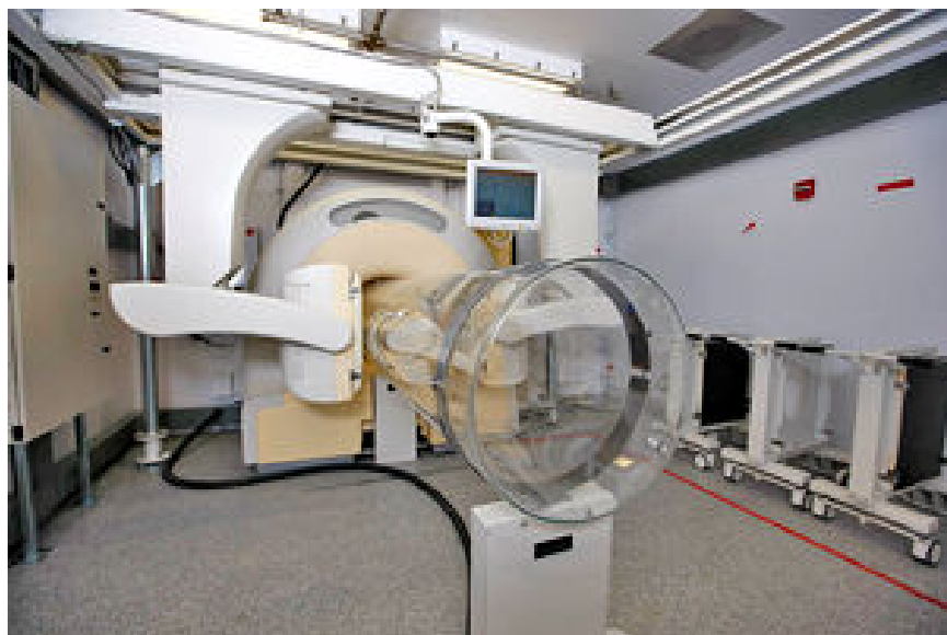
Fig. 4.43.1: Single-photon emission computed tomography (SPECT CT) machine. (Image source National Institute of Allergy and Infectious Diseases (NIAID) and National Institutes of Health) [322].
