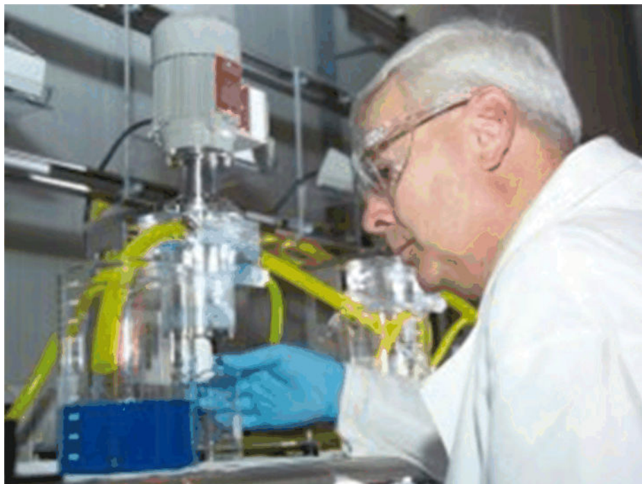
Fig. 4.89.1: The Medical Actinium for Therapeutic Treatment (MATT) is a separations process that recovers ^{225}\text{Ac} from unused nuclear fuel so the isotope can be used in cancer treatment and research. (Image Source: Idaho National Laboratory) [585].
