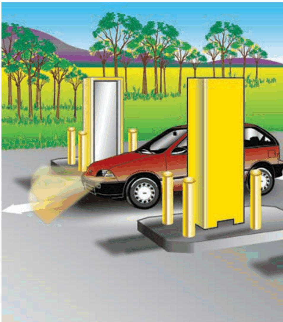
**Fig. 4.2.1:** Radiation detectors are installed in many areas to screen people, vehicles, and cargo for radioactive materials.  $^3\text{He}$  detectors are sensitive to **thermal neutrons** and are used to detect isotopes of uranium and plutonium that might be used in nuclear weapons along with other sources that produce **neutrons** by **radioactive decay**. (Image Source: U.S. Government Accountability Office) [30].
