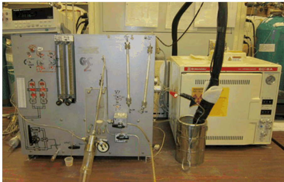
Fig. 4.28.2: Shimadzu GC-8A Gas Chromatograph (GC) with an Electron-Capture Detector (ECD) . (Image Source: The Reston Chlorofluorocarbon Laboratory, U.S. Geological Survey) [230, 231].
